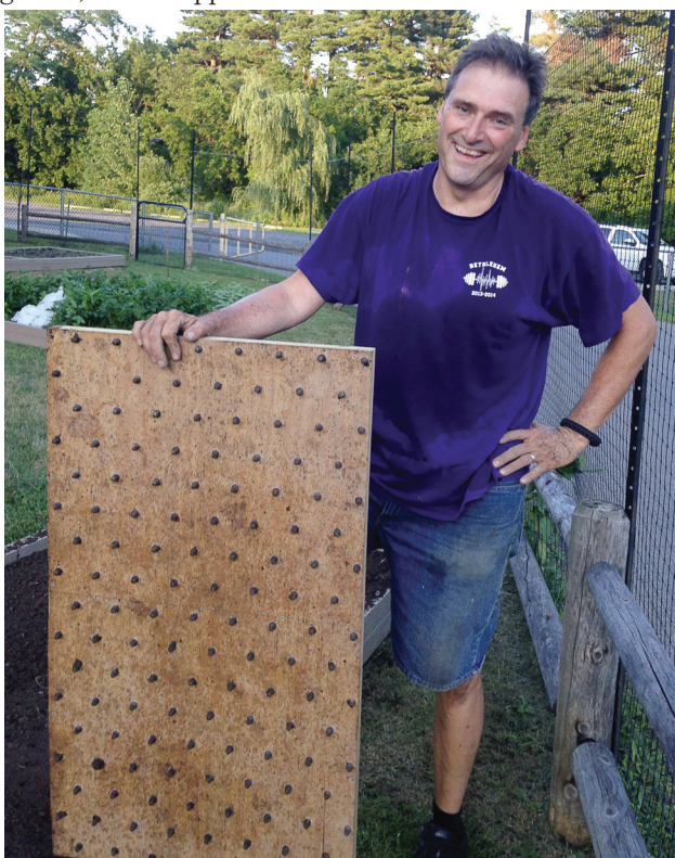
◀ Mark Warford built the carrot dimpler to help small hands plant carrot seeds at a predetermined depth and spacing.
