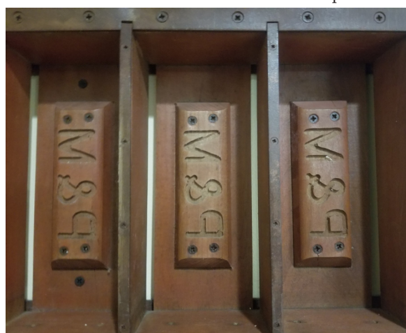
A P&M Brick mold for making molded-clay bricks. This was the standard way in the early years along the Hudson River in Coeymans.
