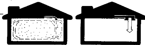
Because Unico System uses aspiration, drafts are eliminated and each room enjoys comfortable, even temperatures.
